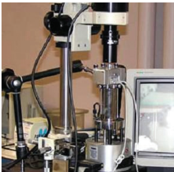
Figure 1: AFM for elasticity measurement.
